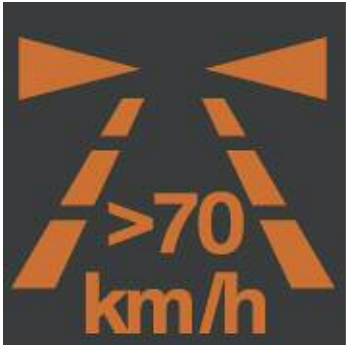
Message indicating the availability of the lane departure warning above 44mph.
