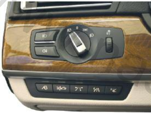
Light switch in position A
