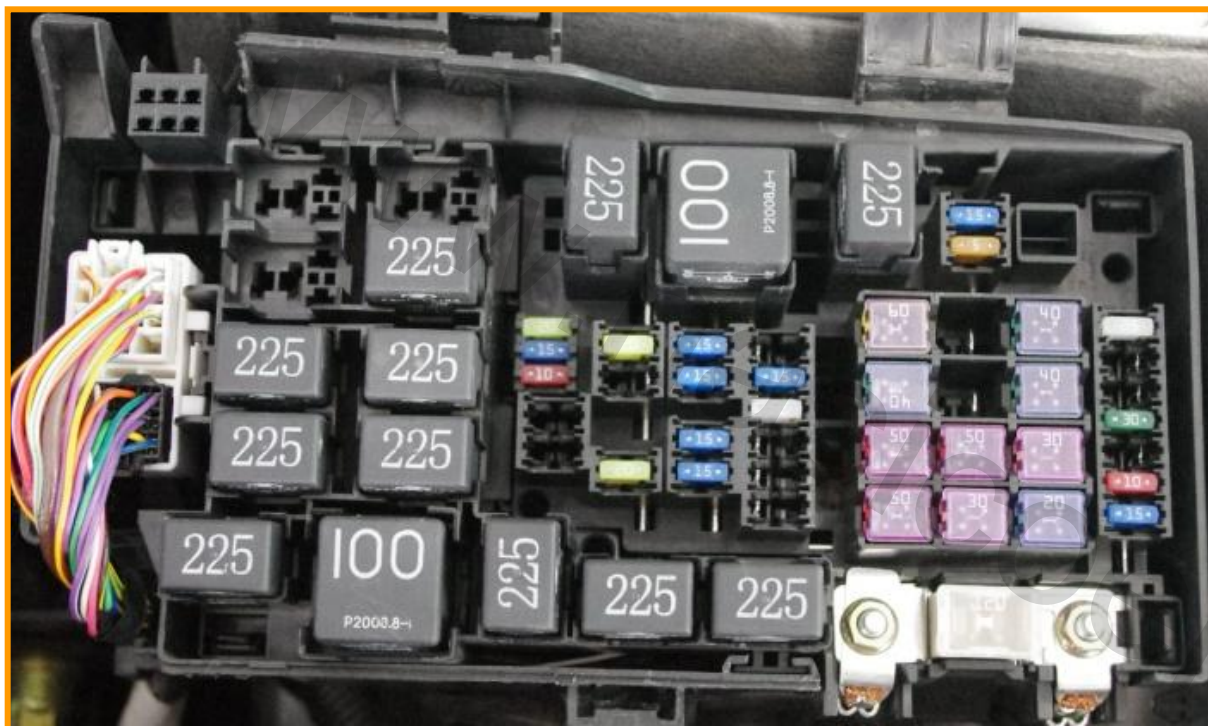
Front hood fuse and relay box
