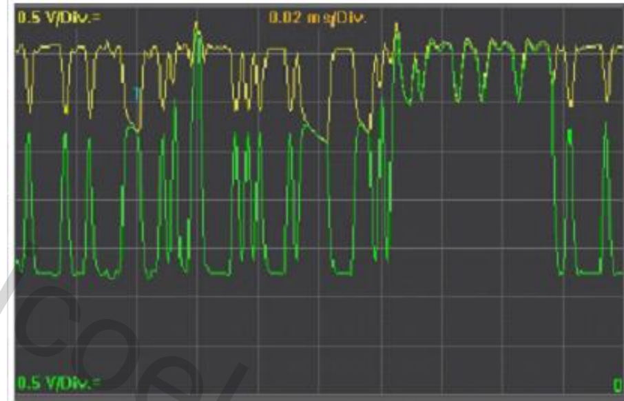
Description of fault: CAN-Low open circuit
