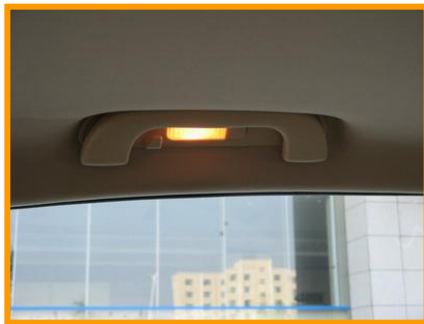
Ceiling handrail light
