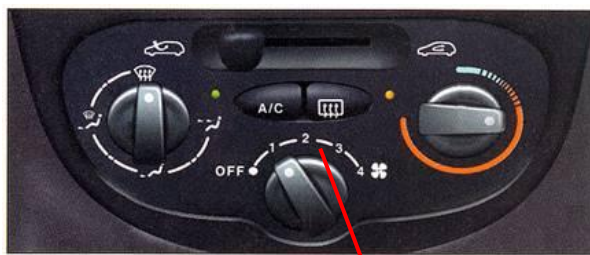
AC / Heater Control Panel
