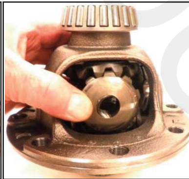
Install the spider gears and washers
