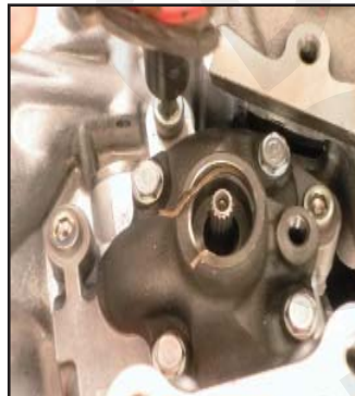
Install new pump seal, install the pump, Torque the inside bolts to 14 Ft. Lbs (19Nm) and outside bolt with o-ring to 20 Ft. Lbs (28Nm)
