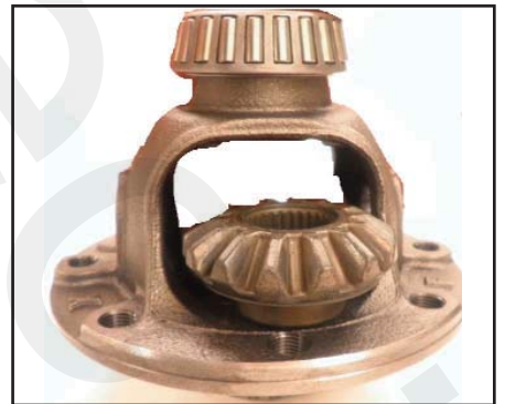
Remove both side gears and washers
