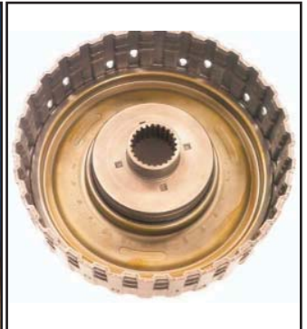
Remove forward clutch balance piston
