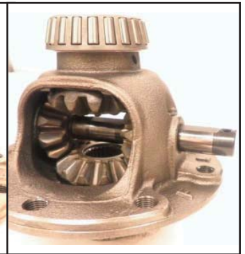
Install spider gear shaft
