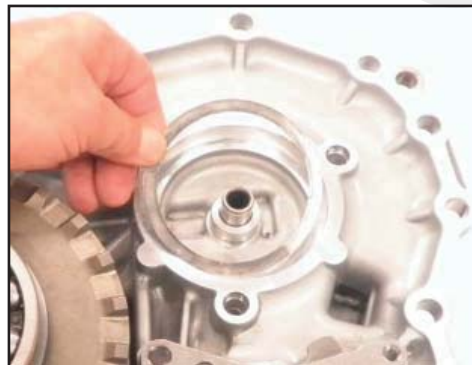
Remove the driven pulley shim
