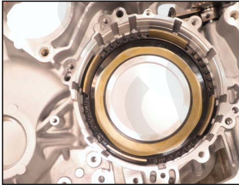
Install reverse clutch piston
