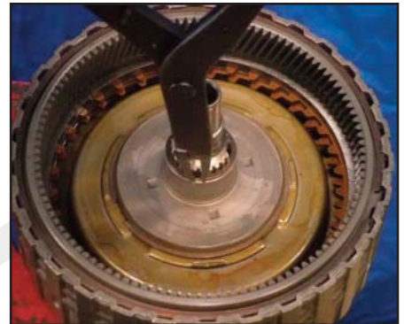
Install input shaft and snap ring
