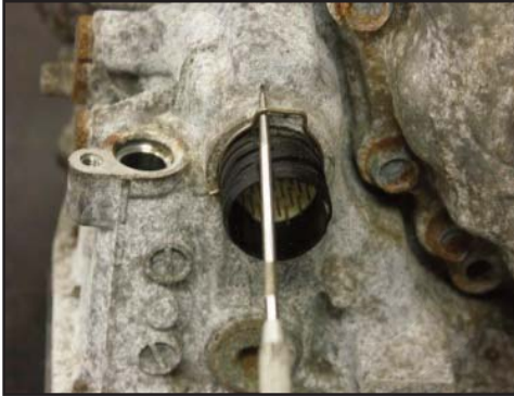
Remove clip holding in case center
