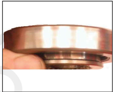
Install the bearing on the secondary shaft with the lip facing down or towards the pulley.
