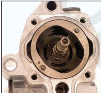
Install pump shaft
