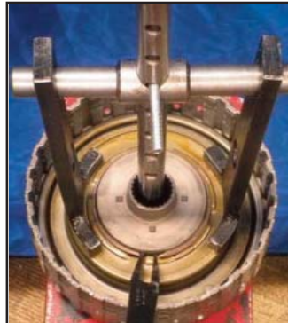
Compress the retainer and remove snap ring
