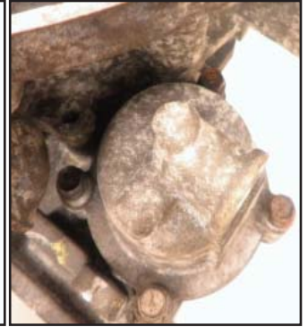
Install cover with new o-ring. Torque bolts to 37 In. Lbs. (4Nm)
