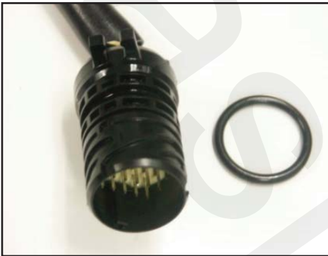
Install case connector into case
