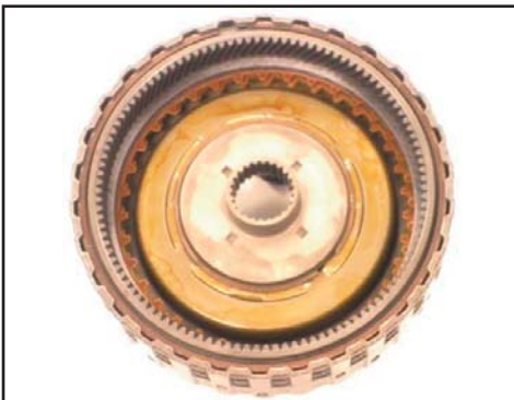
Install ring gear and upper snap ring
