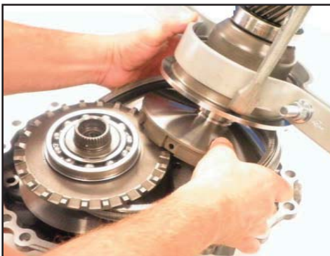
Remove driven pulley
