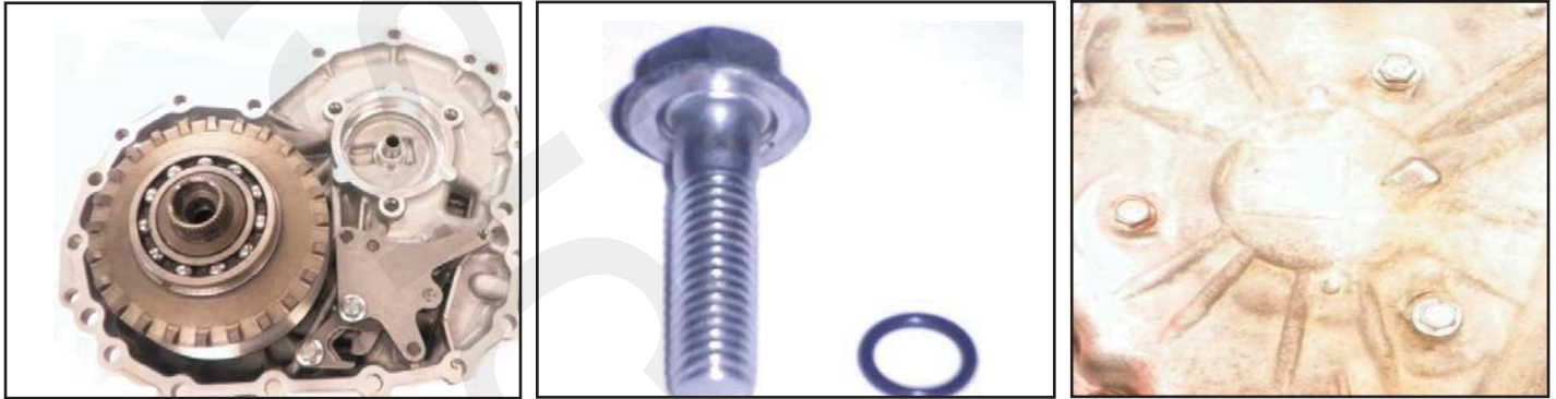
Install primary pulley into the end cover with new o-ring on the bolts. Torque to 33 Ft. Lbs. (45Nm)
