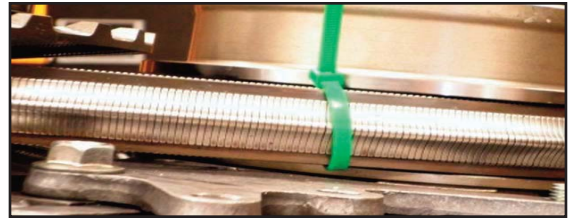
Always wire tie belt, if not, belt could come apart
