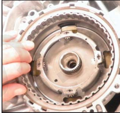
Install torrrington bearing and planet carrier
