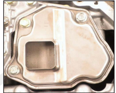
Install filter with new o-ring. Tighten bolts to 70 In. Lbs. (8Nm)
