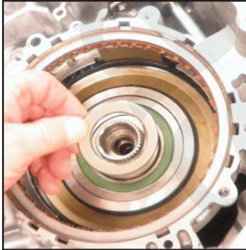
Install torrrington bearing and planet carrier
