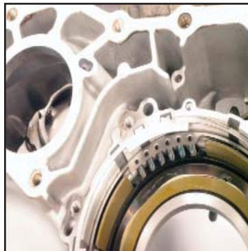
Compress retainer install snap ring
