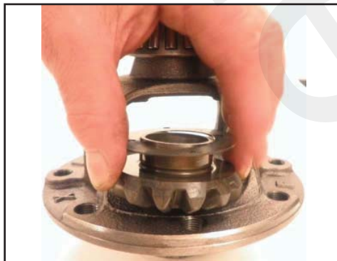
Remove both side gears and washers
