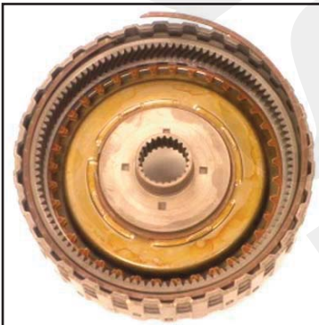
Remove the snap ring and planetary ring gear
