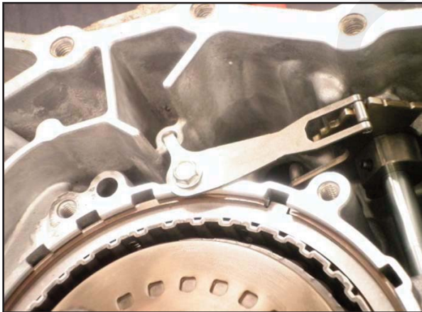
Remove detent spring
