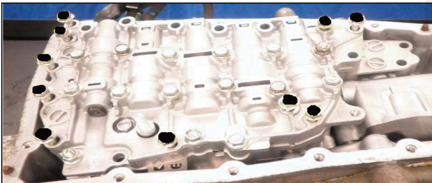
Remove marked bolts to remove valve body.
