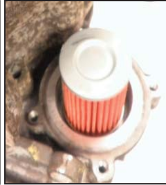
Install cooler filter
