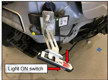
Ensure the metal side is placed against the fixing adapter.
