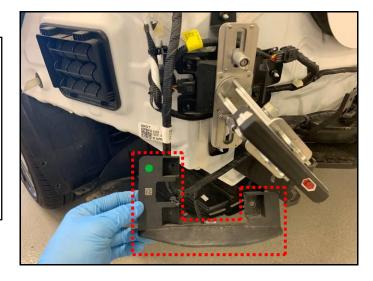
12. Insert the horizontal measuring device, turn the laser ON (select the switch which displays a line), and aim the light to cross the string.
