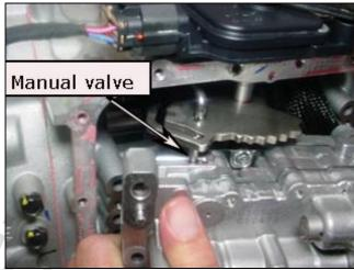
20. Install the valve body bolts and torque the bolts to specification in the order shown.
