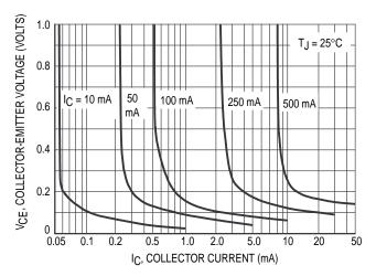
Figure 5. Collector Saturation Region
