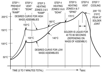
Figure 7. Typical Solder Heating Profile
